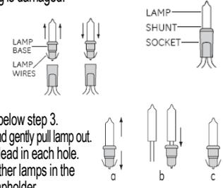
To reduce the risk of overheating replace burned-out lamps promptly. Use 2.5 Volt, 0.425 Watt lamps only.
