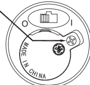
FIG. 1 Unscrew to open the battery compartment cap.
